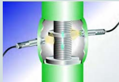
Recognition of the valve position (completely open or closed)
